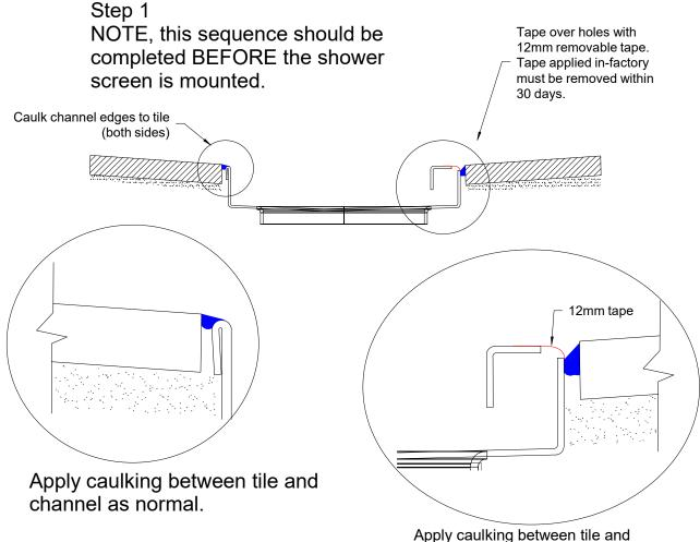
Apply caulking between tile and channel. Any caulk covering tape or drainage holes can be removed by either removing tape, or gently combing caulk off holes.
