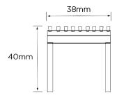
Grates longer than 1500mm supplied in sections. Tile Inserts longer than 1200mm supplied in sections. Channels over 3000mm supplied in sections with joiner. +/-2mm tolerance on
